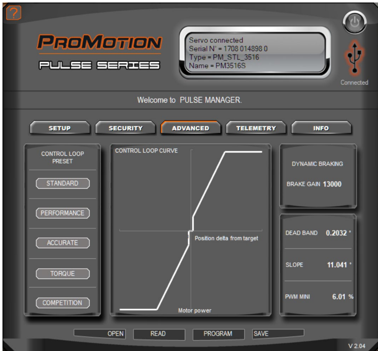
Advanced Setting Screen displays data about the control loop settings.
