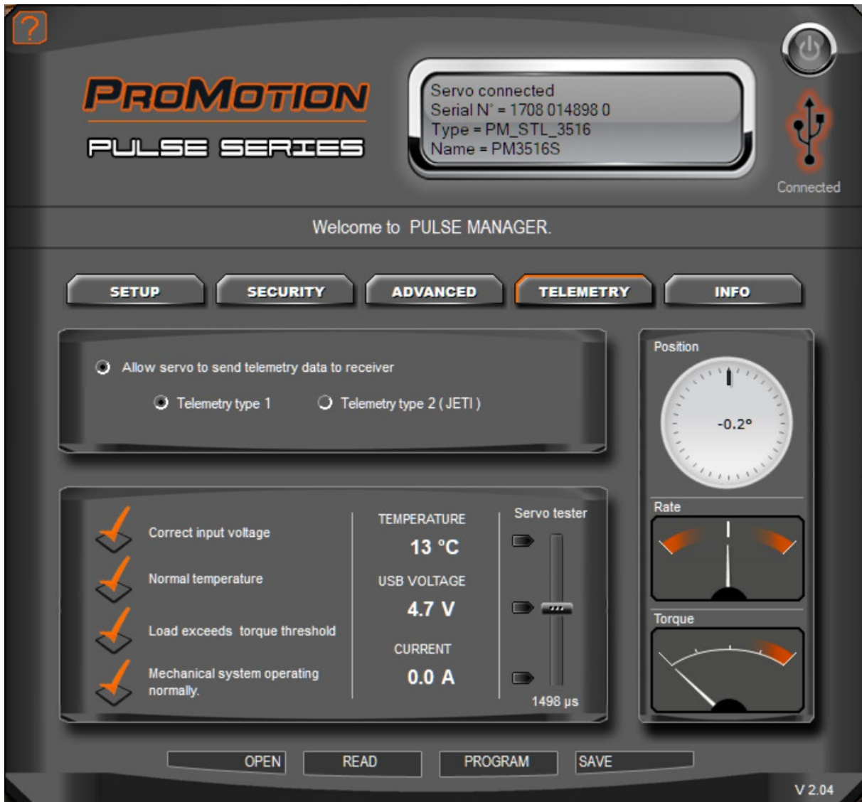
Telemetry screen displays data from the servo.
